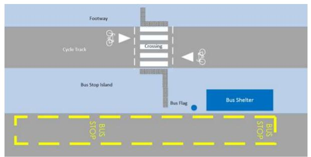
Figure 2 Bus Stop Bypass layout with two-way cycle track and zebra crossing
