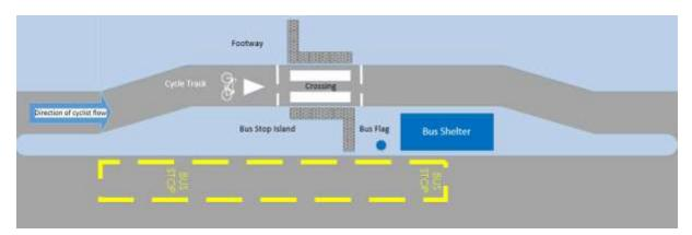
Figure 1 Bus Stop Bypass layout with 1-way cycle track and zebra crossing
